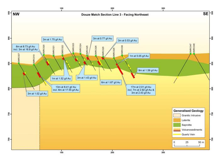
Figure 3: Section across shallow RC drill holes on Line 3
