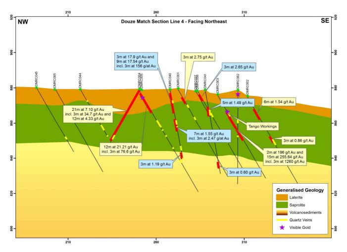
Figure 2: Section across shallow RC drill holes on Line 4
