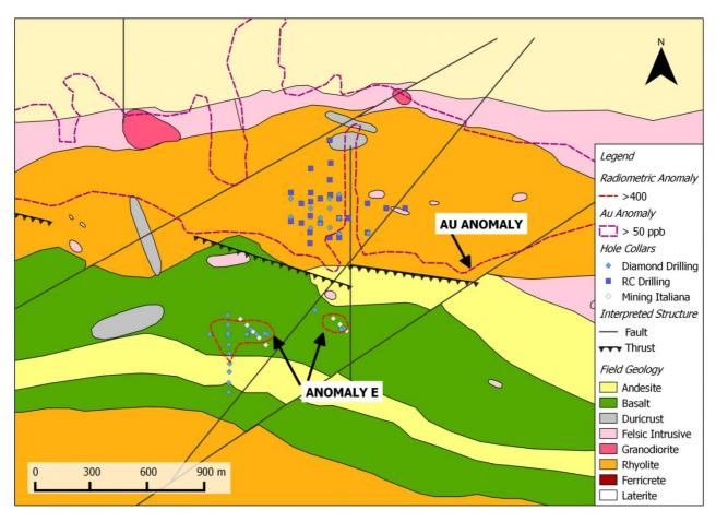
Figure 1: Balatindi Local Geology with Gold Soil Anomaly and Radiometric Anomaly E, and drill collars
